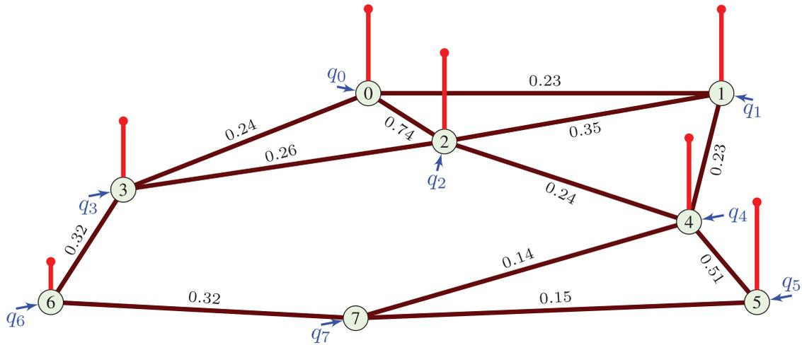
**Figure 6.6:** Temperature,  $x(n) = T(n)$ , as a signal on a heat transfer graph, with  $q_1, q_2, \dots, q_7$ , as the external heat flux values at the corresponding vertices.
