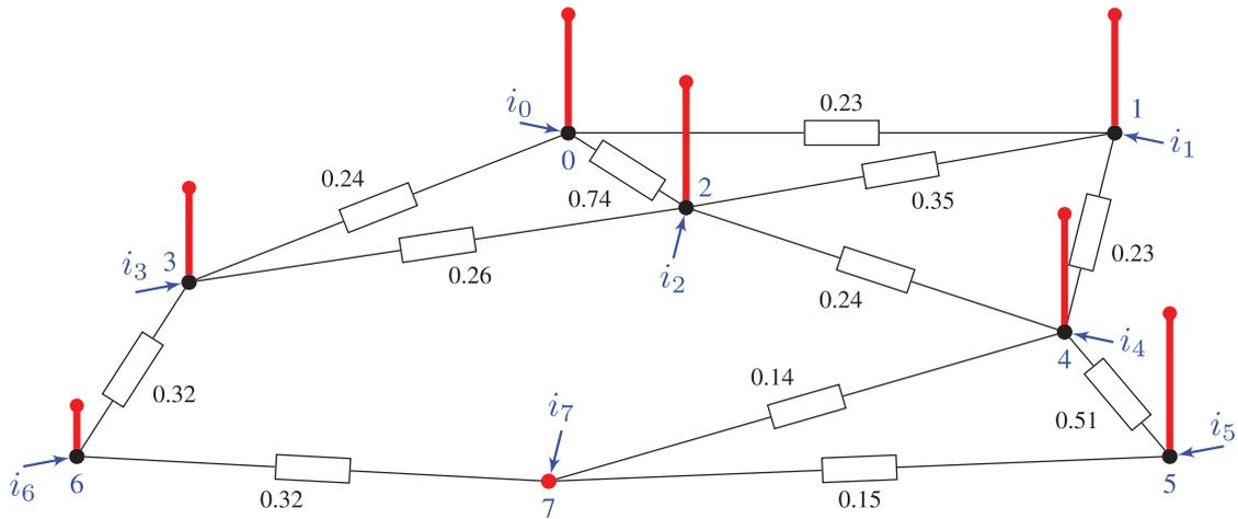
**Figure 6.1:** Electric potential,  $x(n)$ , as a signal on an electric circuit graph.
