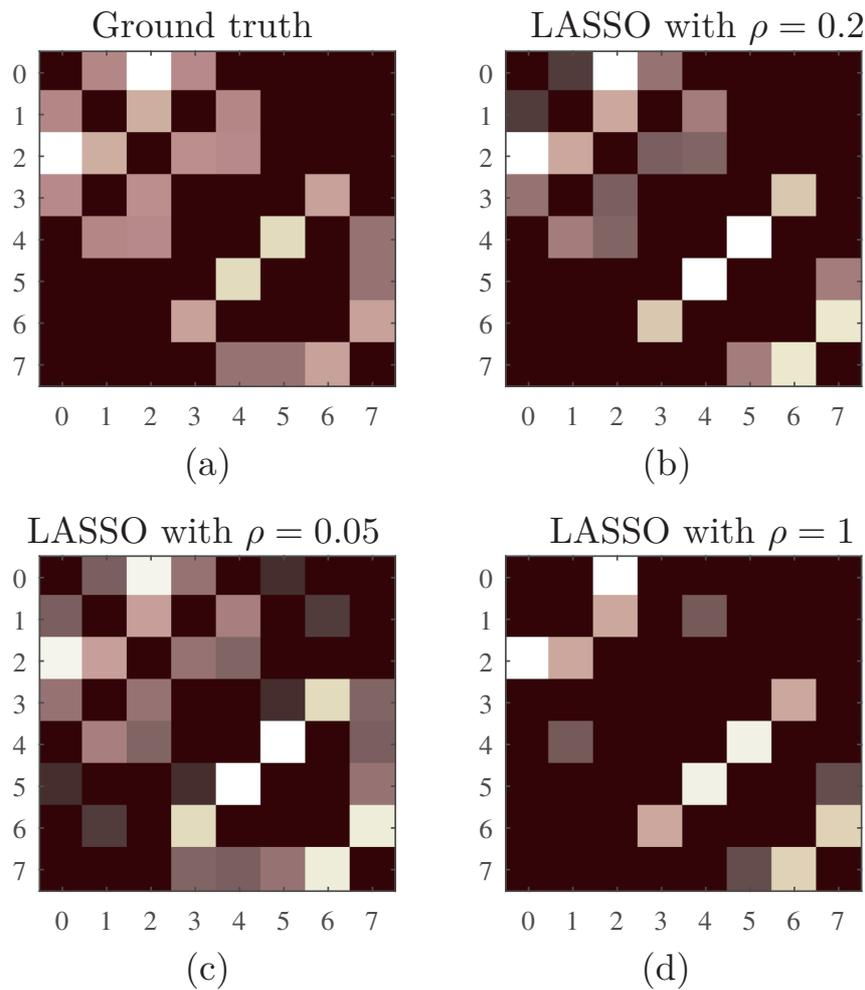
**Figure 4.1:** Estimation of the weight matrix for the graph from Figure 2.2 in Part I with color-coded element values. (a) Ground truth weight matrix. (b) Estimated weight matrix with LASSO and  $\rho = 0.2$ . (c) Estimated weight matrix with LASSO and  $\rho = 0.05$ . (d) Estimated weight matrix with LASSO and  $\rho = 1$ .
