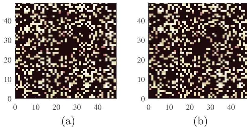
**Figure 4.9:** Estimation of the weight matrix for a graph with  $N = 50$  randomly positioned vertices. (a) Ground truth weight matrix. (b) Estimated weight matrix using sparsity minimization of the normalized Laplacian and the polynomial fitting method.
