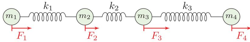
**Figure 6.7:** Spring-mass system on a path graph.
