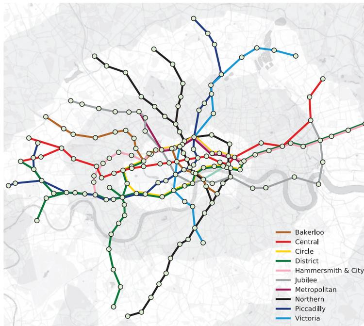
**Figure 12.1:** Graph model of the London underground network in Zones 1–3.
