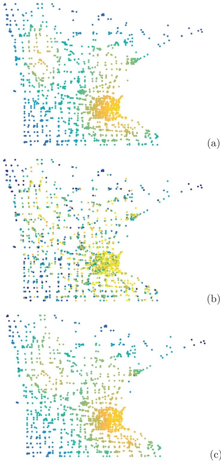
**Figure 2.3:** Temperatures simulated on the Minnesota roadmap graph. (a) Original synthetic temperature field signal. (b) Noisy temperature signal. (c) Low-pass filtered temperature signal from (b). The signal values are designated by the corresponding vertex color.
