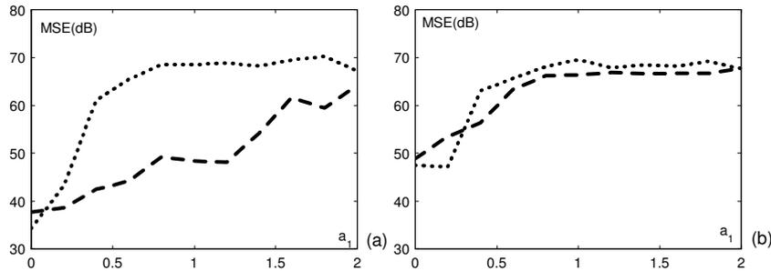
Fig. 3. MSE of the chirp-rate estimation: (a) Impulse noise environment; (b) Mixture of Gaussian and impulse noise. Dashed line - adaptive robust LPFT; Dotted line - adaptive standard LPFT.
