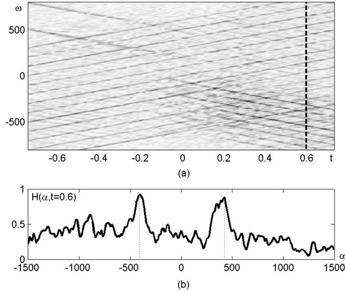
Fig. 4. Multicomponent signals: (a)  $AFT'(t, \omega)$  (instant  $t = 0.6$  is marked with dashed line); (b)  $H(\alpha, t)$  for  $t = 0.6$ .
