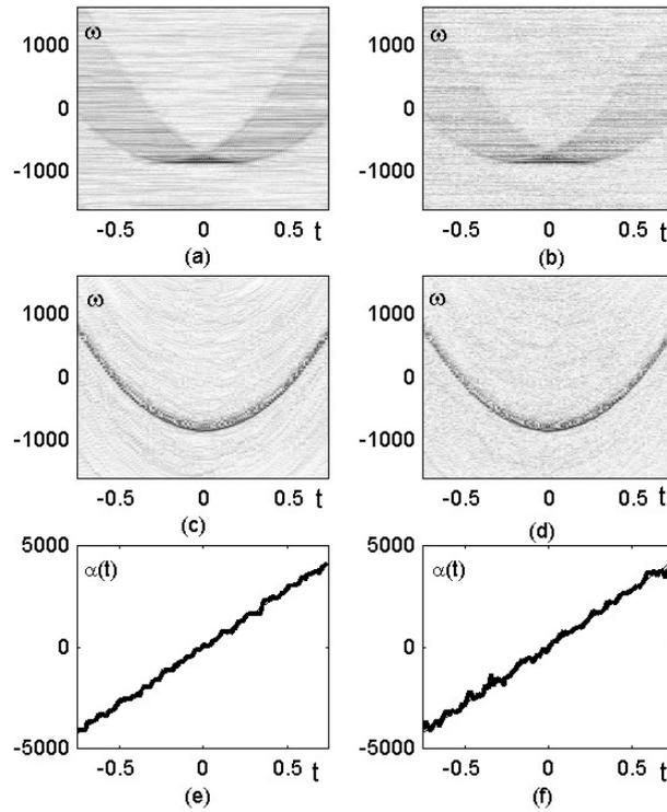
Fig. 2. TF representations of signal embedded in Gaussian noise: (a)  $STFT_S(t, \omega)$ ; (b)  $STFT_{R2}(t, \omega)$ ; (c)  $AFT(t, \omega)$  calculated by the standard LPFT; (d)  $AFT(t, \omega)$  calculated by the robust LPFT; (e) Chirp-rate estimation by using the standard LPFT; (f) Chirp-rate estimation by using the robust LPFT.
