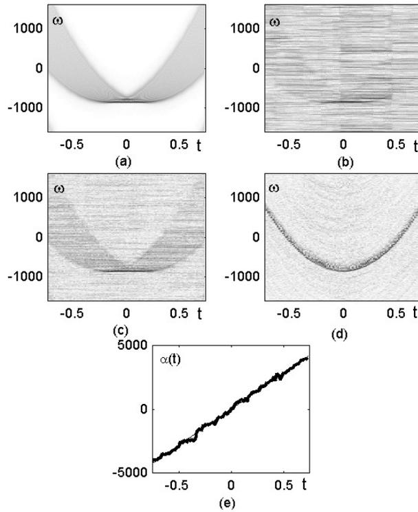
Fig. 1. TF representations of signal embedded in impulse noise: (a)  $STFT_S(t, \omega)$  of non-noisy signal; (b)  $STFT_S(t, \omega)$ ; (c)  $STFT_{R2}(t, \omega)$ ; (d)  $AFT(t, \omega)$ ; (e)  $\hat{\alpha}(t)$ .
